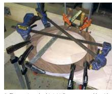
**8.** The steering wheel is initially cut out roughly with a bandsaw from walnut and then assembled and glued up in two laminated layers.
