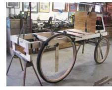
Establishing the correct location for the wheels. Proper steering angles and spring size must be determined, along with resolving a host of other mechanical issues.
