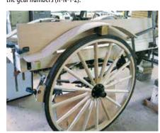
**19.** Test fitting the steam-bent ash-wood fenders to the Daimler truck's body.
