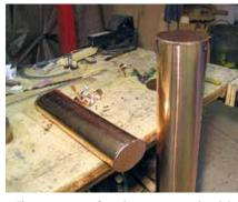
The next step is to form the copper gas tank and then test fit the crimped ends on both tanks prior to soldering them both tight.
