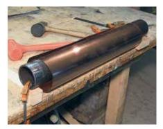
**4.** Rolling the copper sheeting for the rear water reservoir by forming it around a section of large diameter metal pipe. Crude perhaps, but it works!
