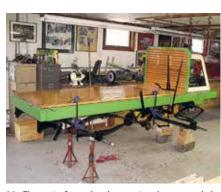
**20.** The main frame has been painted green and the varnished red-oak rear bed is installed. Did I forget something? Oh, yeah. Where's the driver's seat?
