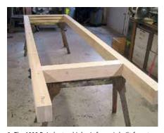
**1.** The 1898 Daimler truck's basic frame is built from two 2x6 beams of laminated poplar, the same wood used in the construction of early Concord stagecoaches.
