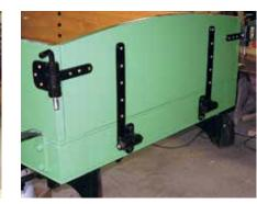
**21.** Getting near the end of construction now, sorting out some final details; closeup of the rear tailgate with hefty strap hinges and matching side-pin latches.
