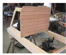
**7.** The finished dashboard is installed on the passenger side of the plywood bulkhead. Note initial test placement of the transmission and clutch.
