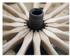
**14.** All of the wheel spokes dovetailed and inserted into the Amish-made metal axle hub in preparation for being bolted through the metal wheel hub.
