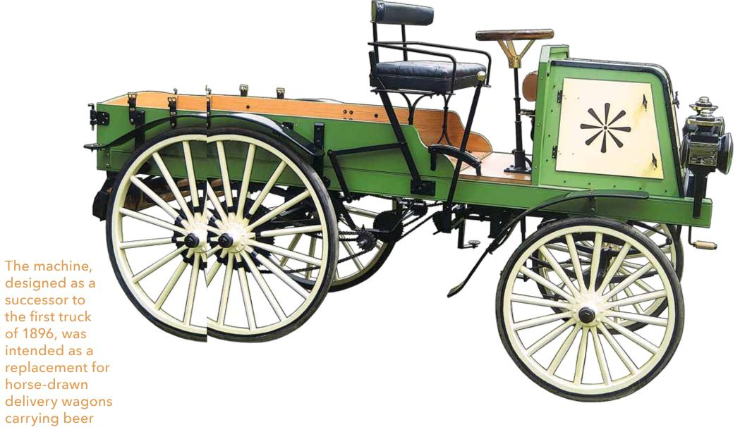
Craftsmen from the Amish community near Eggers's Connecticut home supplied handmade buggy leaf springs, metal-edged wheel rims, metal wheel hubs and leather upholstery.
