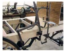
**17.** Positioning, attaching and connecting up the 1898 replica's two small stagecoach-style shoe brakes.
