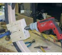
**12.** Drilling the Amish-made metal-edged wooden wheel rims to accept the wooden spokes, using basic geometry and a shop-made drilling jig.
