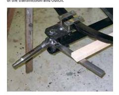
**10.** In this view, potential front axle and steering problems are shown in the process of being ironed out. The tie rod measurements are also taken at this time.
