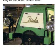
**23.** Front end of the truck with the brass Daimler nameplate (cut with a laser) and two single-candle headlights installed. Note replica engine crank and flywheel.
