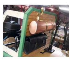
**22.** Closeup of the truck's finished dashboard with the leather glove compartment, copper gas tank and bronze oil-pressure gauge installed.
