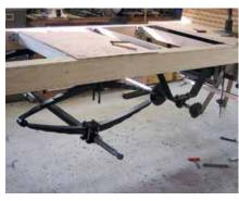
11. Next, the rear leaf springs (buggy springs made by Amish craftsmen) and axle are bolted in place beneath the truck's body.
