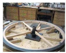
**13.** Installing the first wooden spokes into the wooden wheel rims and axle hubs. Ash wood was a traditional material choice from which to make wagon-wheel spokes.
