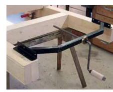
**3.** Fitting the fabricated metal brace to stiffen the front end, act as an engine mount and locate the engine crank.
