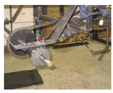
**15.** Drive chains and chain sprockets had to be tested in conjunction with the engine to ensure the arrangement would transmit the proper speed to wheels.
